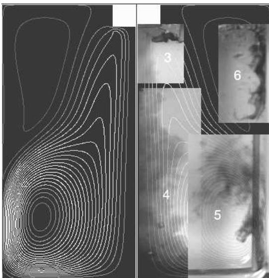
Figure 5: Left, CFD streamlines in a beaker ( $d=125$  mm) Right, ink experiments. The numbers represent observations 3-6 from table 3
